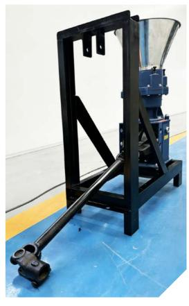
Tractor PTO Driven it Operates Efficiently Delivers High Output
